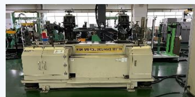
<RR Compound Torsion Beam Axle (CTBA) Fatigue Test>
